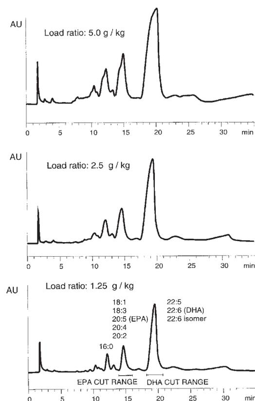
**FIG. 1.** Supercritical fluid chromatograms from preparative fish oil ethyl ester injections at different column load ratios. Fraction collection intervals for docosahexaenoic acid (DHA) and eicosapentaenoic acid (EPA) concentrates are indicated. Kromasil 10-C18, 10 × 250 mm column. Pressure, 145 bar. Temperature 65°C. Mobile-phase linear velocity 1.9 mm/s. AU refers to absorbance units from the ultraviolet detector.
