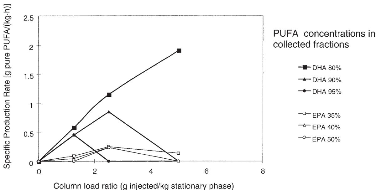
**FIG. 2.** The effect of column loading on the specific production rate of polyunsaturated fatty acids (PUFA) at different purities. Calculated from results obtained in Step 2 preparative SFC experiments. See Figure 1 for abbreviation.
